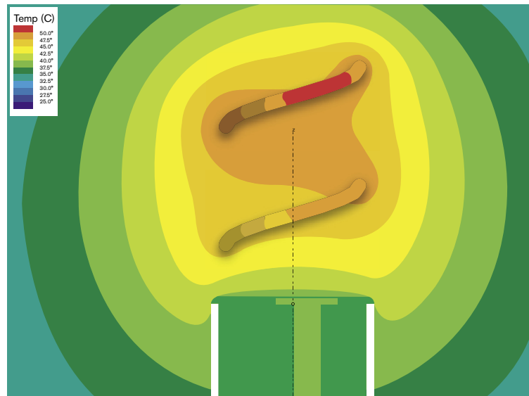
Figure 3 – Temperature profile from mathematical modeling of active fixation pacemaker lead in an MRI field.
